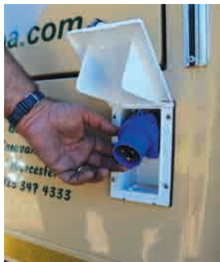
FAR LEFT Simply release the pop-up roof catches to open the roof. The gas struts make this so much easier. LEFT The blue Fredlin plug connector.
